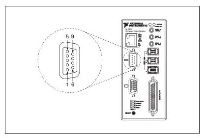
Figure 3-7. COM1 DSUB 9-Pin Connector
